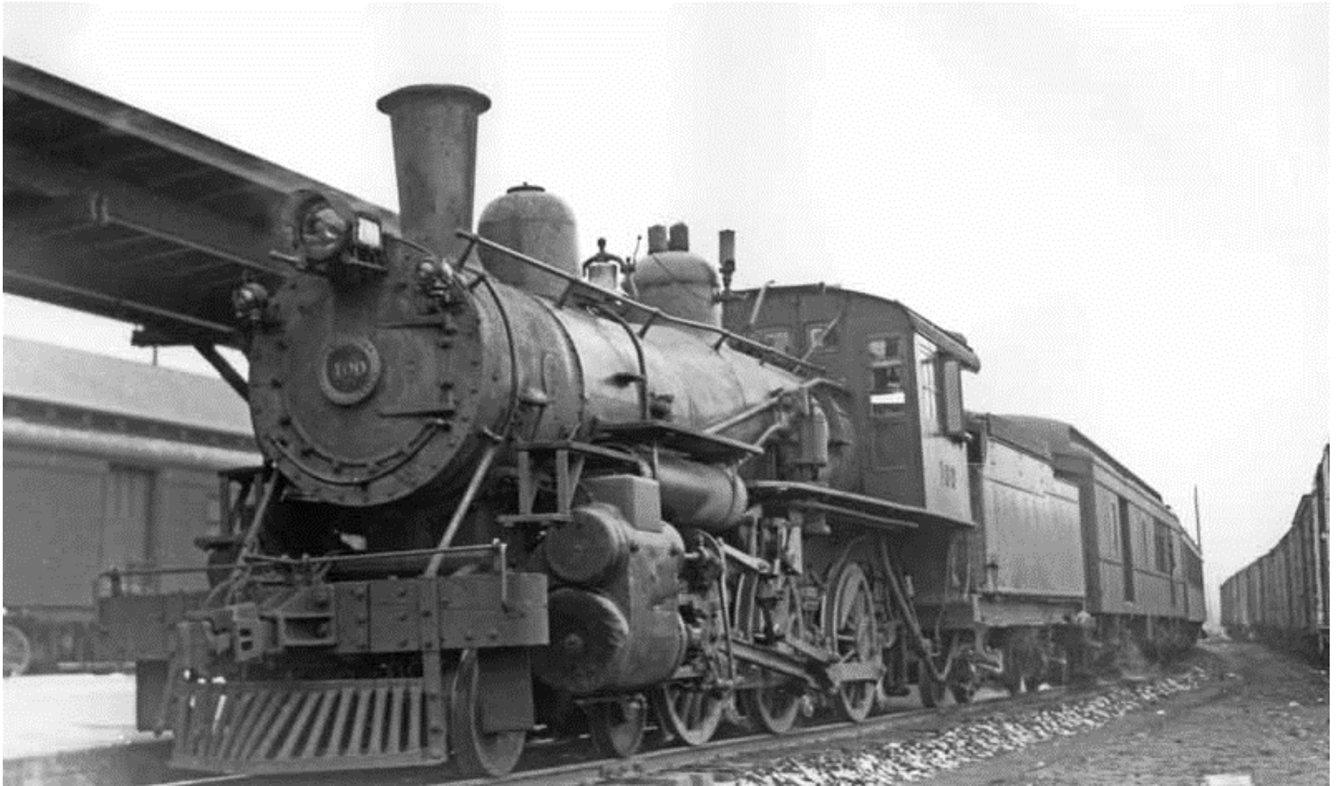
Figure 29. “Southbound [passenger] train 38 with Class G-2 locomotive 100 at Johnson City, Tn. Some locomotives fans said the class G-2 was ‘quaint’. Others said it was ‘plain ugly’. Circa 1930.” Another source dates this photograph to 2 February 1935. “H.W. Painter/G.W. Best – Floyd Bruner Collection”. 59 This train appears to be at the Clinchfield depot. Engine #100, a Baldwin 4-6-0 Ten-Wheeler, was built in December 1908, with an empty weight of 82 tons. Based on the available photographs, it appears that the Clinchfield employed their Ten-Wheelers in passenger service. This engine was retired on 1 September 1938 and scrapped.
