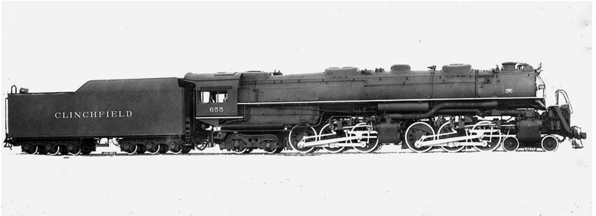
Figure 5. “4-6-6-4 Challenger steam locomotive No. 655 – After the 2-8-8-2s Clinchfield turned to the single-expansion 4-6-6-4 type during World War II. Also built eight to a Delaware & Hudson design in 1942-43; an additional four in 1947 were CRR’s last steam locomotives. Engine 655 was from the first order.” 8 Engine #655, an American 4-6-6-4 Challenger, was built in January 1943, with an empty weight of 303½ tons. Based on previous Clinchfield practice, it was probably used to haul coal trains This engine was retired on 1 May 1954.
