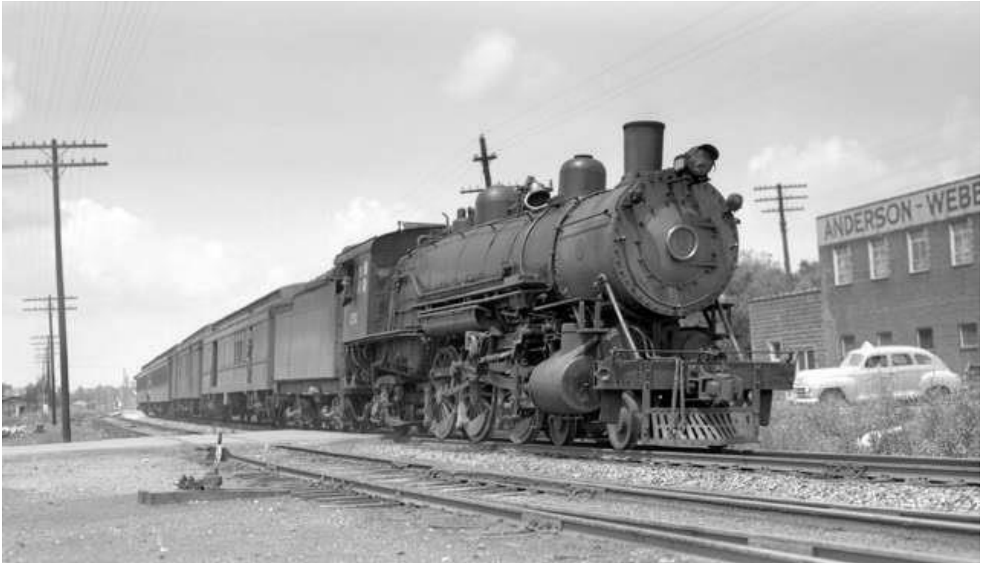
Figure 26. “Clinchfield Engine 151” pulling a passenger train. 56 Engine #151, a Baldwin 4-6-2 Pacific, was built in June 1910, with an empty weight of 117½ tons. The Clinchfield employed Pacific type engines in passenger service north of Erwin, Tennessee. This engine was retired on 22 June 1951 and scrapped. Note the “Anderson-Webb” building, this company was a wholesaler of eggs, butter and cheese. It was in business by 1949. The author has not found any sources that document where this building was located.
