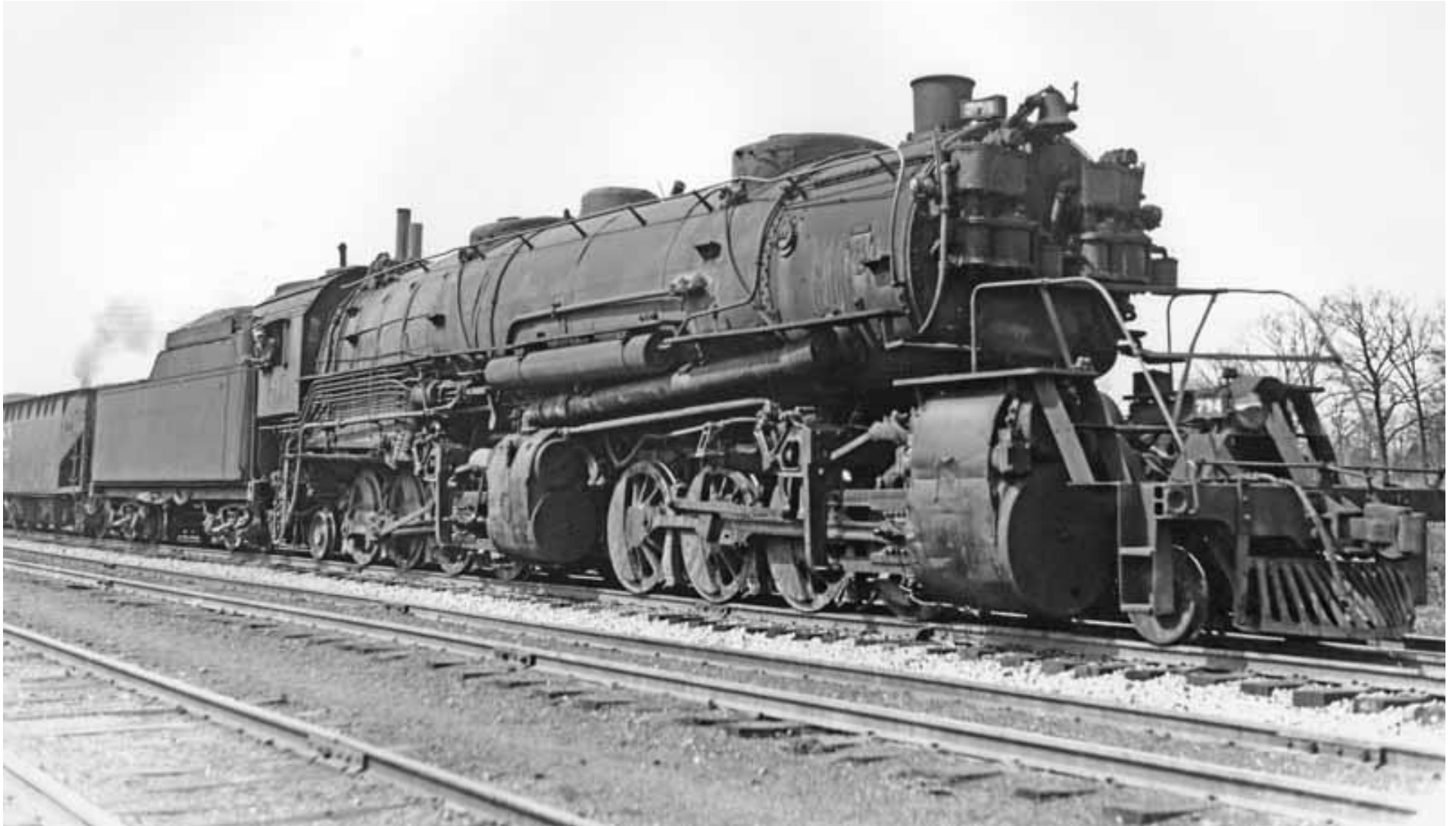
Figure 2. “Clinchfield 734 2-8-8-2 At Johnson City, TN 3-46”. 5 Engine #734, a Baldwin 2-8-8-2 Chesapeake (Clinchfield Class L-2), was built in November 1919, with an empty weight of 270½ tons. L-2 Class locomotives were used on “Slow Freight Trains (Third Class)... The slow freight trains are, for the most part, composed of coal cars. They are made up at Dante, southbound, and are operated as through freights to Erwin... Either one L-2 or an L-3 Mallet locomotive is used on each of these trains between Erwin and Dante, except on southbound trains an L-1 Mallet engine is used on the rear from Kingsport to Unicoi, 6 miles north of Erwin. The maximum load is 100 cars.” This engine was retired on 1 September 1952.
