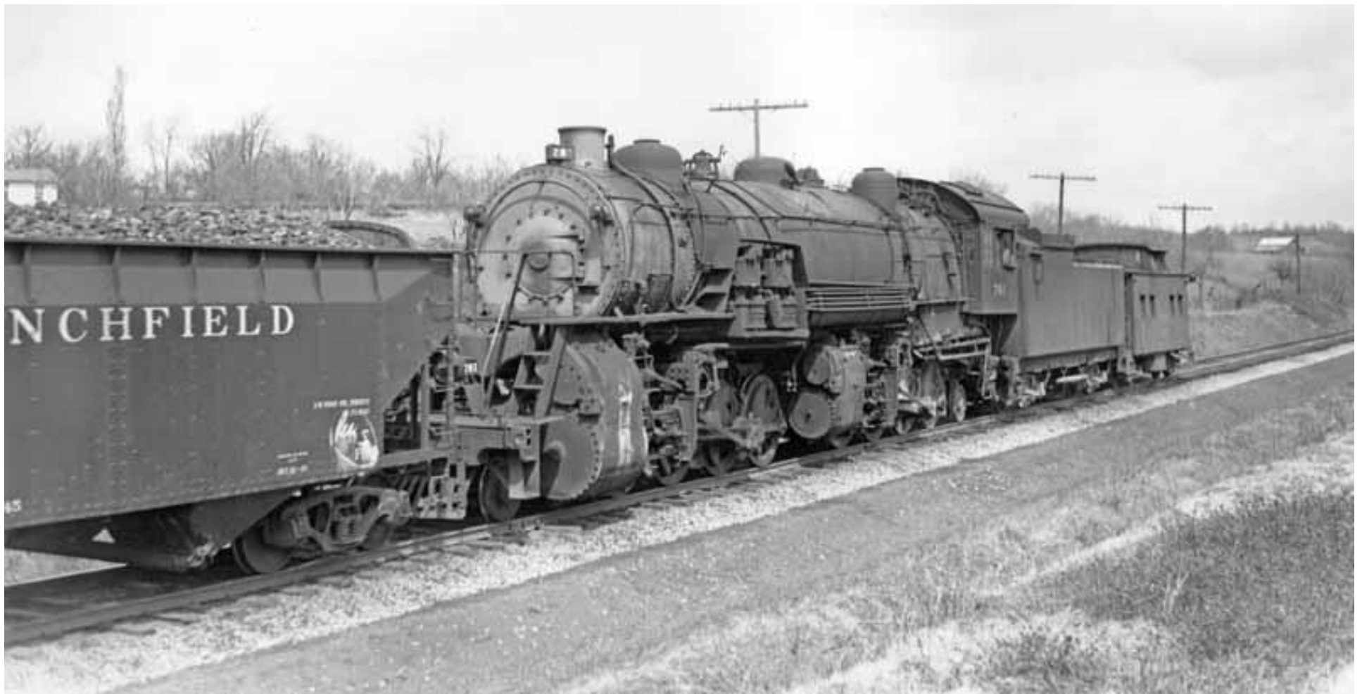
Figure 4. "Clinchfield 701 2-8-8-2 pusher on SB coal train Johnson City, TN 3-46". 7 Engine #701, a Baldwin 2-8-8-2 Chesapeake (Clinchfield Class L-1), was built in March 1919, with an empty weight of 262 tons. Based on previous Clinchfield practice, it was probably used to haul coal trains This engine was retired on 18 August 1950.
