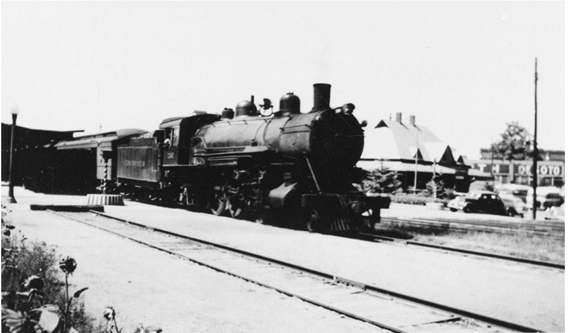
Figure 28. "Clinchfield Engine with ET&WNC Depot in the Background, Johnson City, TN". 58 A southbound passenger train waits at the Clinchfield depot, with what appears to be a 4-6-2 Pacific (P-1 Class) engine at its head. The P-1 Class was retired in 1951, so this photograph appears to date from the late 1940s or early 1950s.
