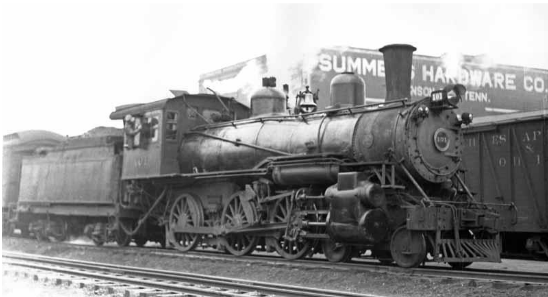
Figure 30. “Clinchfield 101 Johnson City, TN 2-2-35” with a passenger train. 60 Note the Summers Hardware building in the background, which indicates that Engine #101 is near the Clinchfield depot in Johnson City. Engine #101 (Clinchfield Class G-2), a Baldwin 4-6-0 Ten-Wheeler, was probably built in December 1908 or later, with an empty weight of 82 tons. Based on the available photographs, it appears that the Clinchfield employed their Ten-Wheelers in passenger service. This engine was retired on 1 September 1938 and scrapped.
