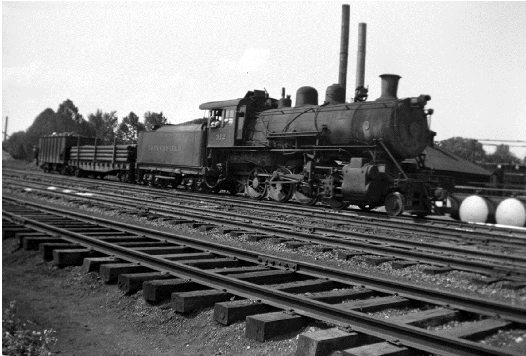
Figure 36. “Clinchfield No. 312 Bemberg”. However, it does not appear that this photograph was taken at Bemberg; note the four parallel standard gauge tracks in the foreground. Perhaps, this was taken adjacent to the Carnegie Addition, on the northside of Johnson City. 70 Engine #312 was a Baldwin 2-8-0 Consolidation (Clinchfield Class H-4). It was built in February 1909, with an empty weight of 100 tons. It appears that the Clinchfield employed their H-4 Class Consolidations primarily as switcher, helper and local freight engines. It was retired on 31 July 1951 and scrapped.
