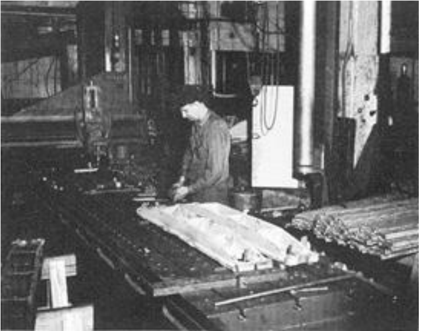
Figure 20. “A machinist prepares a casting for finishing operations on a planing mill.” This photograph was published in 1959. 44
