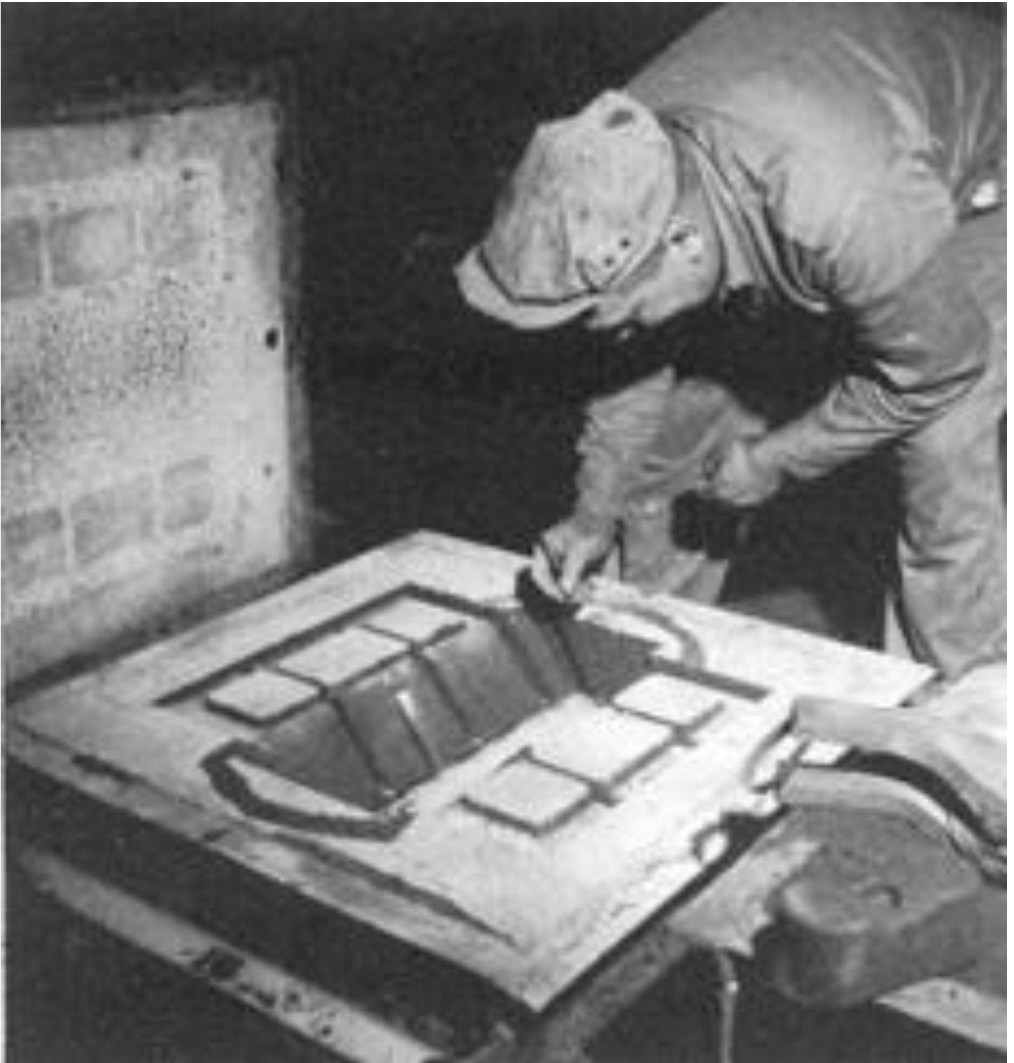
Figure 17. “A moulder fashions the intricately detailed pattern into which molten metal will be poured to solidify in the shape of the mold.” This photograph was published in 1959. 41
