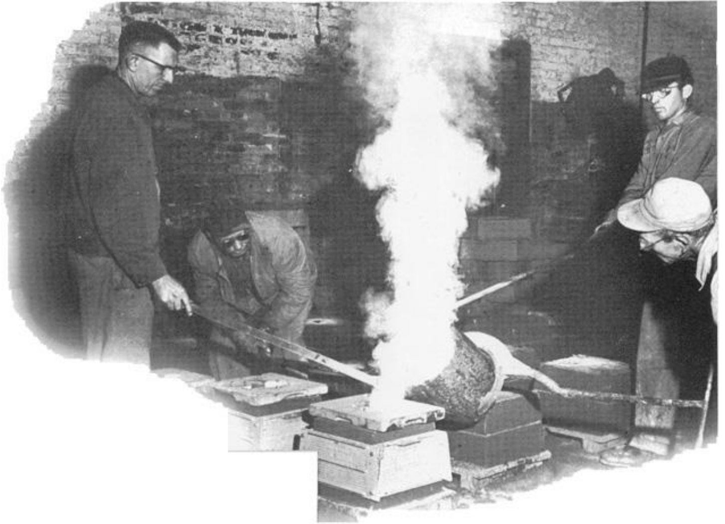
Figure 18. “Foundry workers pour melted aluminum into a mold under the direction of V.M. Eads (left), foundry foreman.” This photograph was published in 1959. 42
