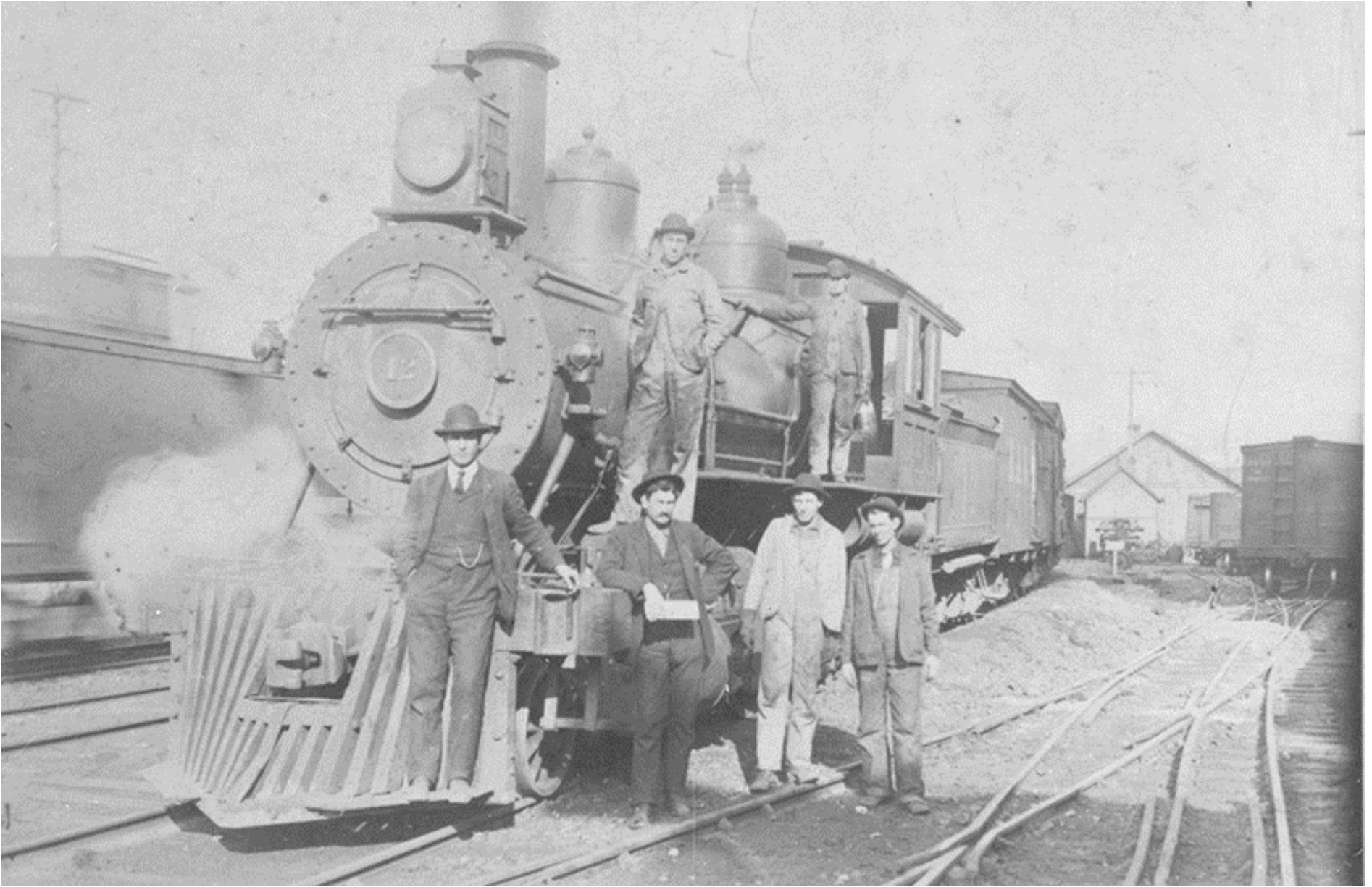
Figure 19. "Southern Railway 2-8-0 No. 12 is parked with a freight train at the ET&WNC interchange track in Johnson City. This engine was originally built for the Richmond & Danville by Schenectady in 1887. Very faint SOUTHERN lettering is on the cab and a large 12 is on the tender. This engine was not scrapped until 1928. Courtesy Jack Williams Collection." 48 Note the dual gauge trackage on the right. This photograph dates to after 1900.
