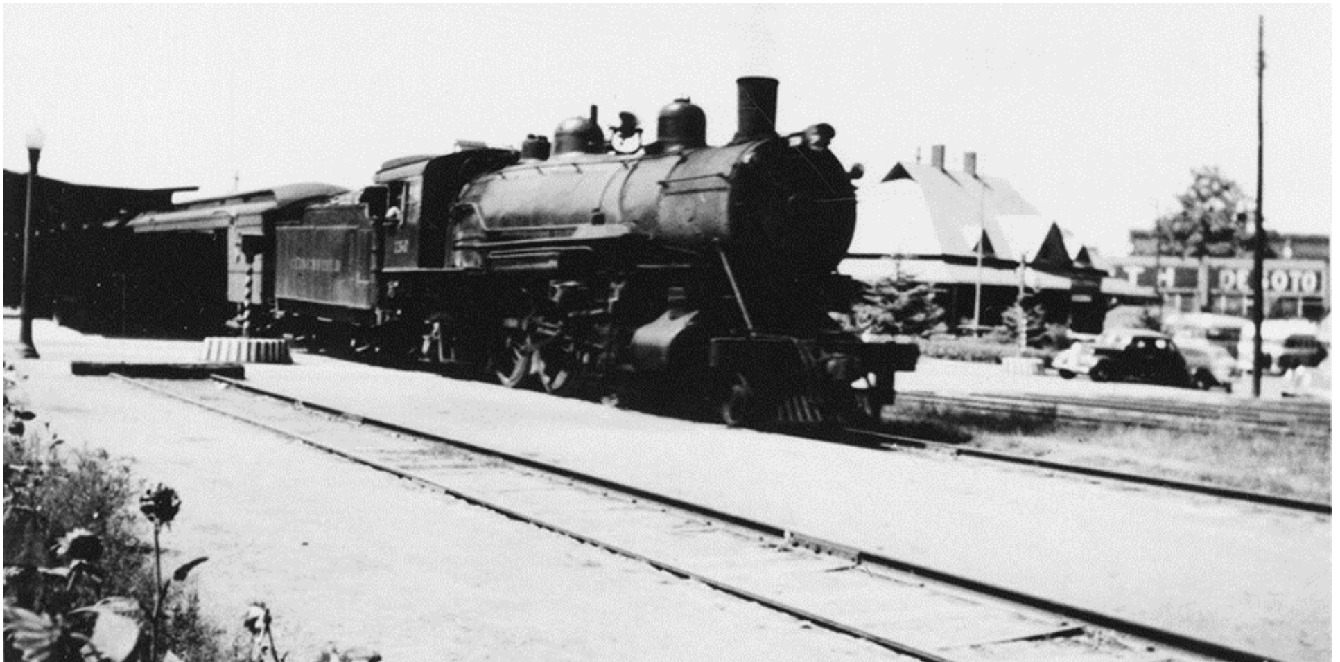
Figure 8. “Clinchfield Engine with ET&WNC Depot in the Background, Johnson City, TN”. 33 A southbound passenger train waits at the Clinchfield depot, with what appears to be a 4-6-2 Pacific (P-1 Class) engine at its head. The P-1 Class was retired in 1951. Note that the dual-gauge trackage that remains in place near the E.T. & W.N.C. depot is somewhat overgrown. “In September 1946, the third rail between Johnson City and Elizabethton was removed”, thus, this photograph predates 1946. 34
