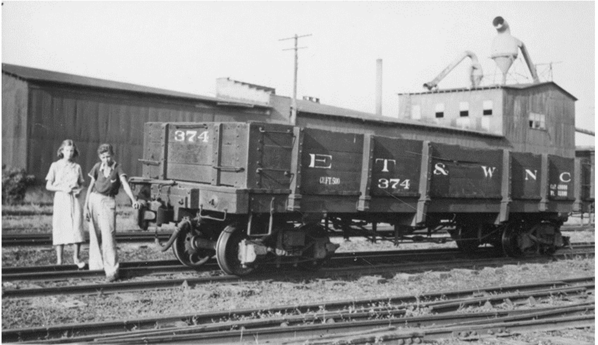
Figure 56. "Gondola #374," by the Harris Manufacturing Company. 162 The dual gauge trackage indicates that this photograph was taken in 1946 or earlier. Note the change in configuration of the cyclone on the roof of the building on the right, in comparison to figures 54 and 55. This change had been made by 13 October 1937. 163
