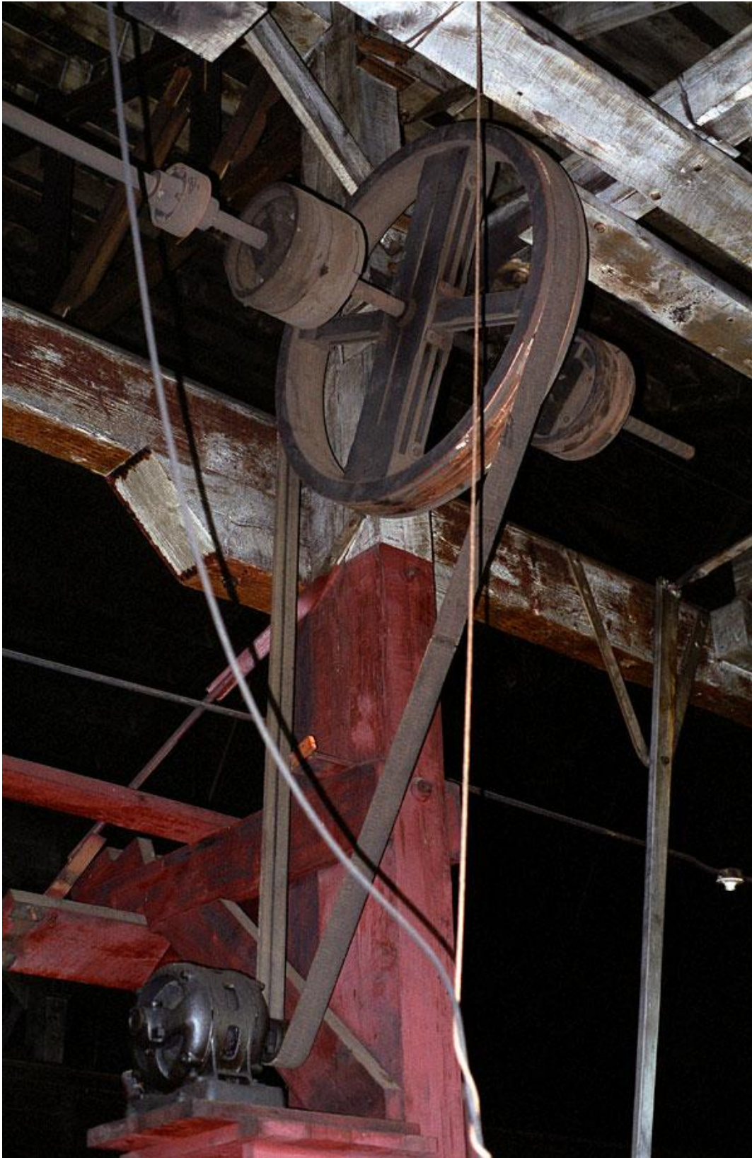
Figure 62. Chris Ford wrote of this photograph: “June 2000... Here’s one of the main belt-driven wheels in the back of the engine house. It looks like its made from laminated wood, and it still works. Don’t think it would have had an electric motor turning it when it was put in, though. Unfortunately, most of the machines tied to these belts are gone.” 73
