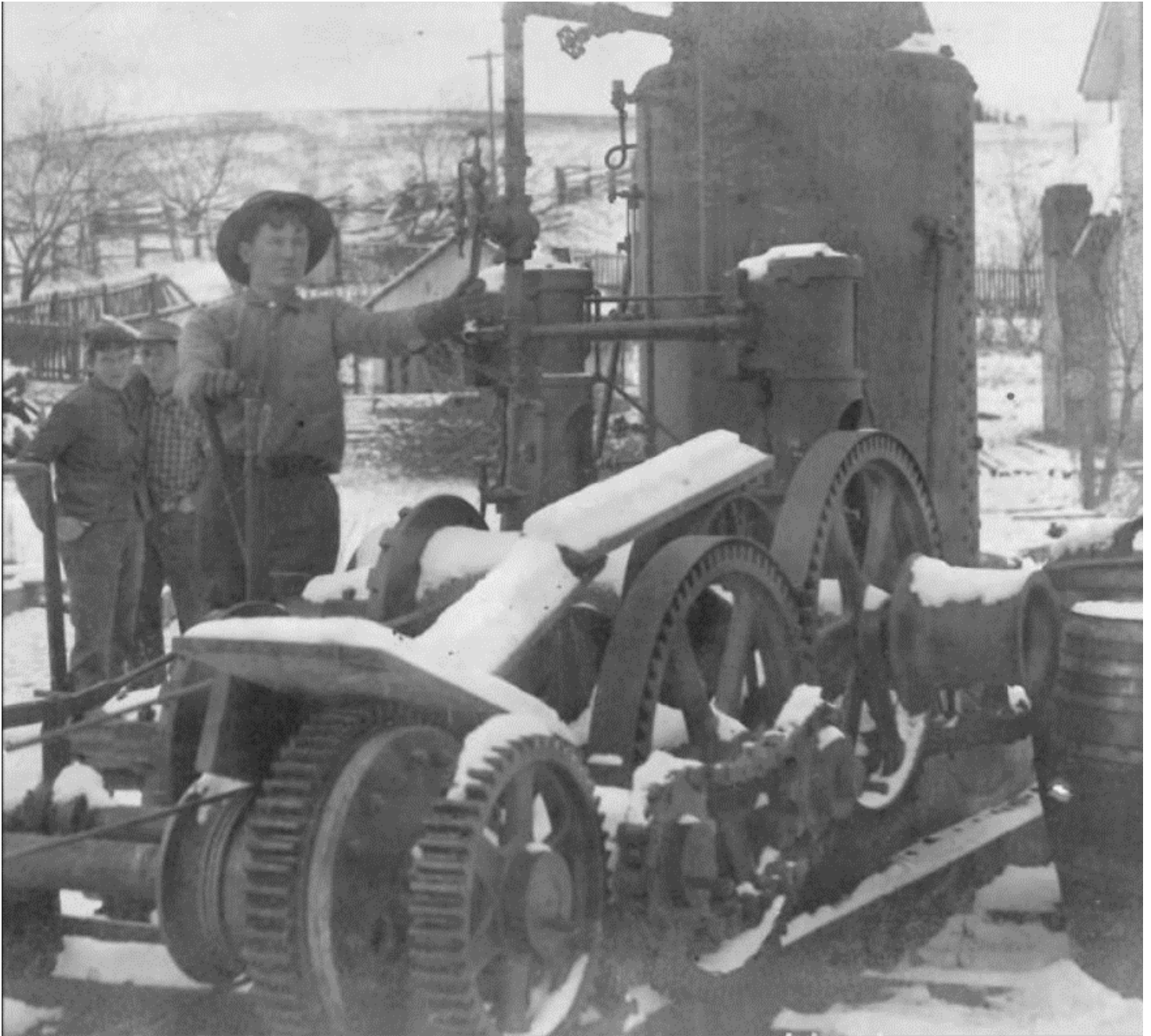
Figure 14. “Steam Donkey. A steam donkey is a steam-powered winch invented in 1881 by John Dolbeer that revolutionized 19 th -century logging in areas with difficult or steep terrain and large logs beyond the capability of a team of oxen or horses. The operator was referred to as a donkey puncher. This postcard was postmarked 1908 in Johnson City and mailed to Polly Dunn in Vaughtsville, Johnson County, Tennessee. At that time, there were 8 lumber wholesalers and 12 lumber manufacturers listed in the city directory.” 56
