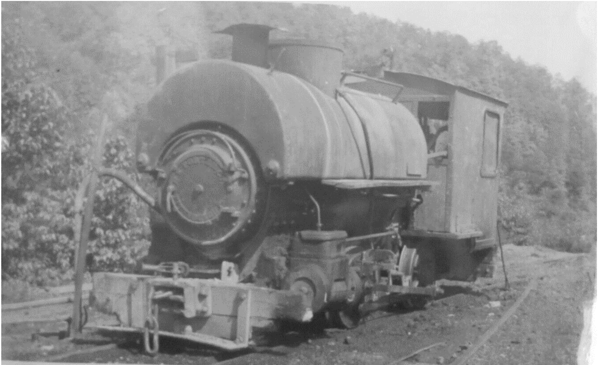
Figure 38. “Johnson City Brick & Tile Co. 2, 3’... Johnson City, Tenn. 8 – 38”. 175 Note that this locomotive appears to be listed as engine #2 and as being 3-foot gauge. Also note that “Johnson City Brick & Tile Co.” appears to be a case of mistaken identity for Johnson City Shale Brick Corporation, see Figure 39.
