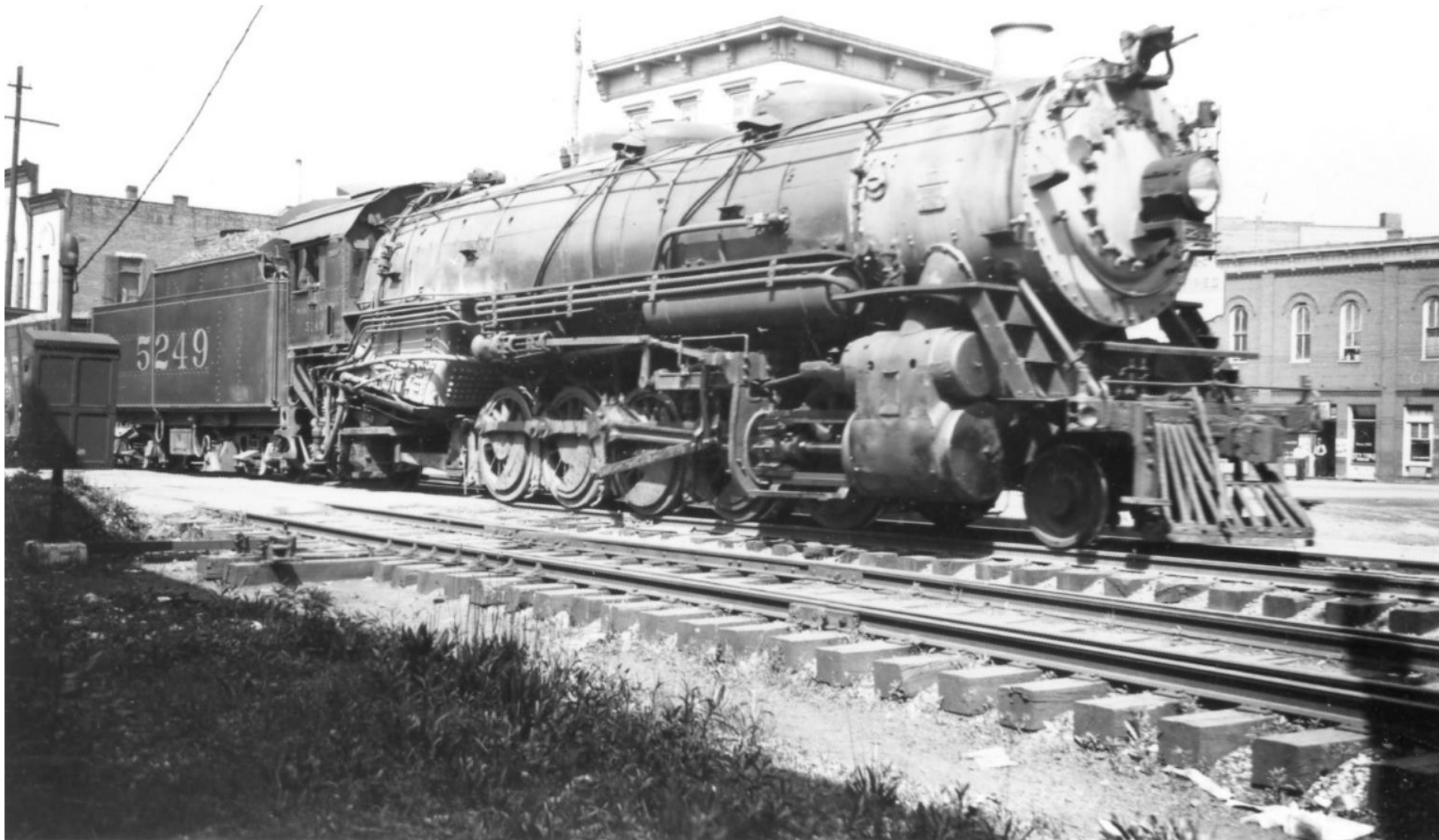
Figure 10. Southern Railway #5249 (with a 2-10-2 “Santa Fe” wheel arrangement) on 18 May 1933. The structure on the right is the William Harr Building, the structure above the engine is the top of the Free Service Tire Company building, and the structure on the left is the W.O. Phillips building. Note that the Western Hotel, which would have been visible between the Free Service Tire Company building and the W.O. Phillips building, had been removed in 1927. 17 See Map 6A.
