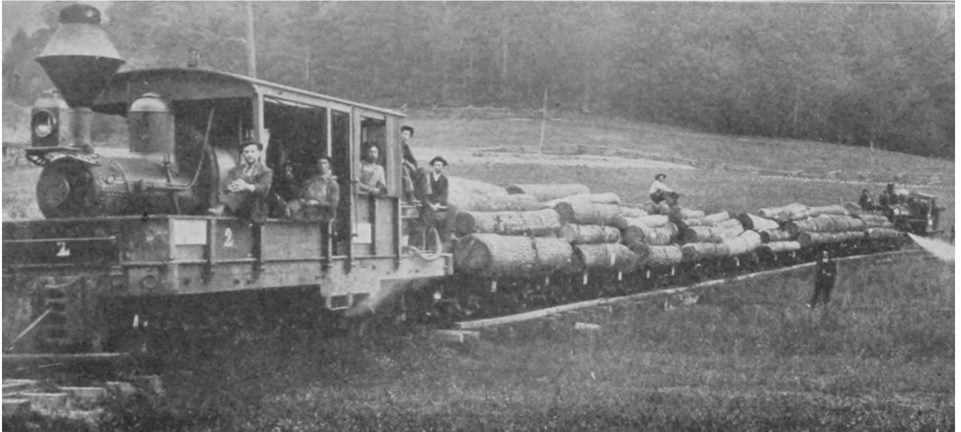
Figure 6. “Log Train En Route to the Mill at Abingdon, Va., [Photo] From the Whiting Manufacturing Company.” American Lumberman , 15 January 1910. 12 Historian Thomas Fetters captioned this photograph: “This is Whiting Manufacturing Company’s No. 2 Class-A Climax (one of two ‘Black Satchels,’) hauling a string of log cars on their Cold Spring operation in Tennessee. This 3-foot gauge 18-ton engine was built in 1906. Their No. 1, a [20-ton] Class-B Climax [shop number 608], built about 1905, brings up the rear...” 13 The Whiting Manufacturing Company based out of Abingdon, Virginia, actually operated five Class A Climaxes, each weighing 18 or 20 tons, one of the 20-ton Climaxes may have been acquired by the Sanford & Treadway for its operation based out of Newland, North Carolina. This photograph and the three below are included to give some indication of what the Sanford & Treadway 20-ton Class A Climax may have looked like. 14
