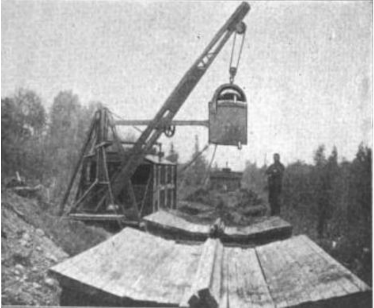
Figure D – 3. “Raymond Gasoline Loader with shovel attachment, now owned by Fountain-Campbell Lumber Co., Ladysmith, Wis. No logging concern is complete without a Raymond combination Log Loader and Excavator.” 125
