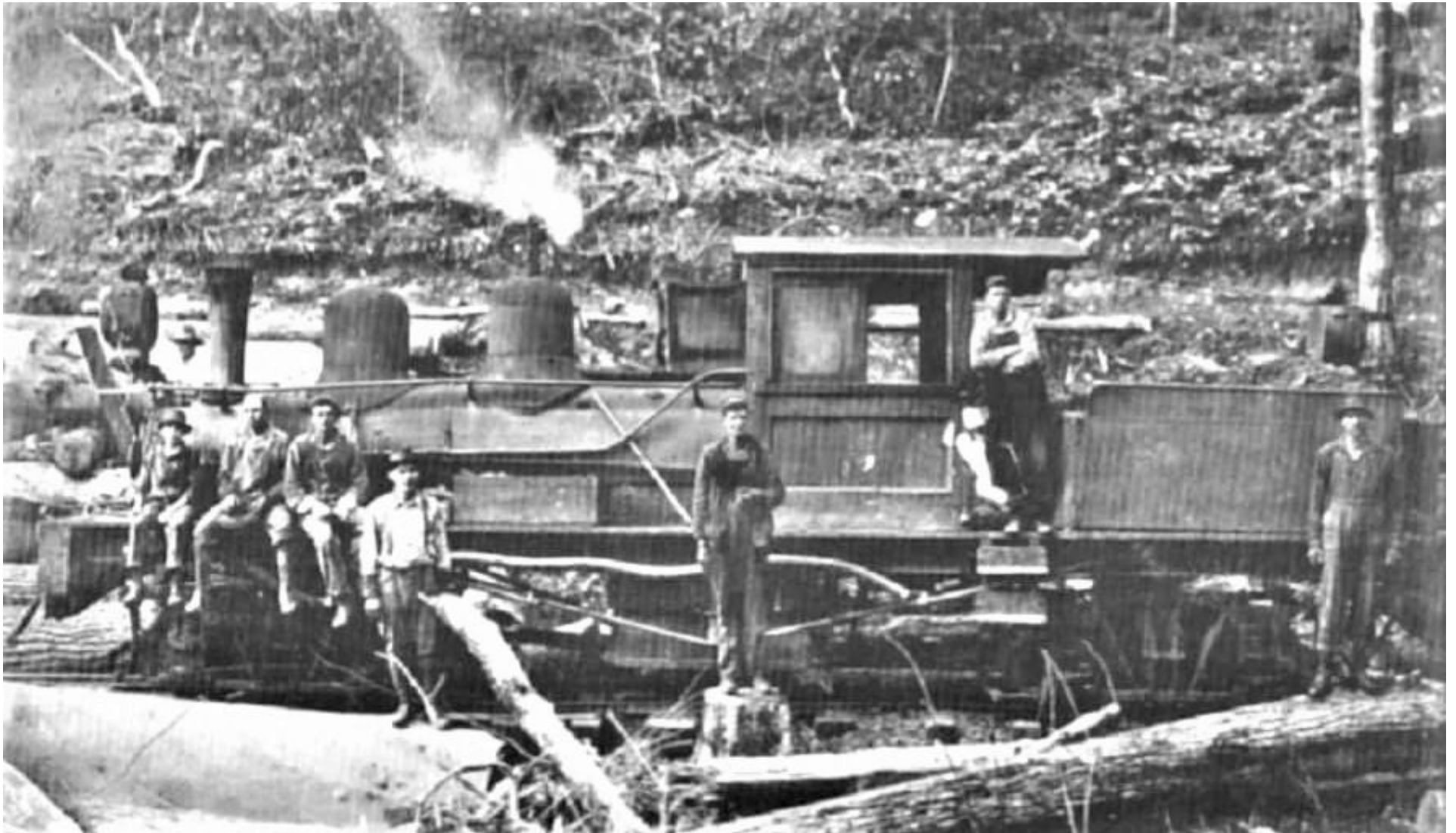
Figure 14. "The W.G. McCain Lumber Company of Butler, Tenn. operated this three-foot gauge 1909 Lima Shay [s/n 2131] which posed with the crew at the millsite. In 1929 this engine was transferred to the D&H MacRae Lumber Company at Linville, North Carolina along the ET&WNC mainline. (Collection of Tom G. King, Kingsport, Tenn.)" 72
