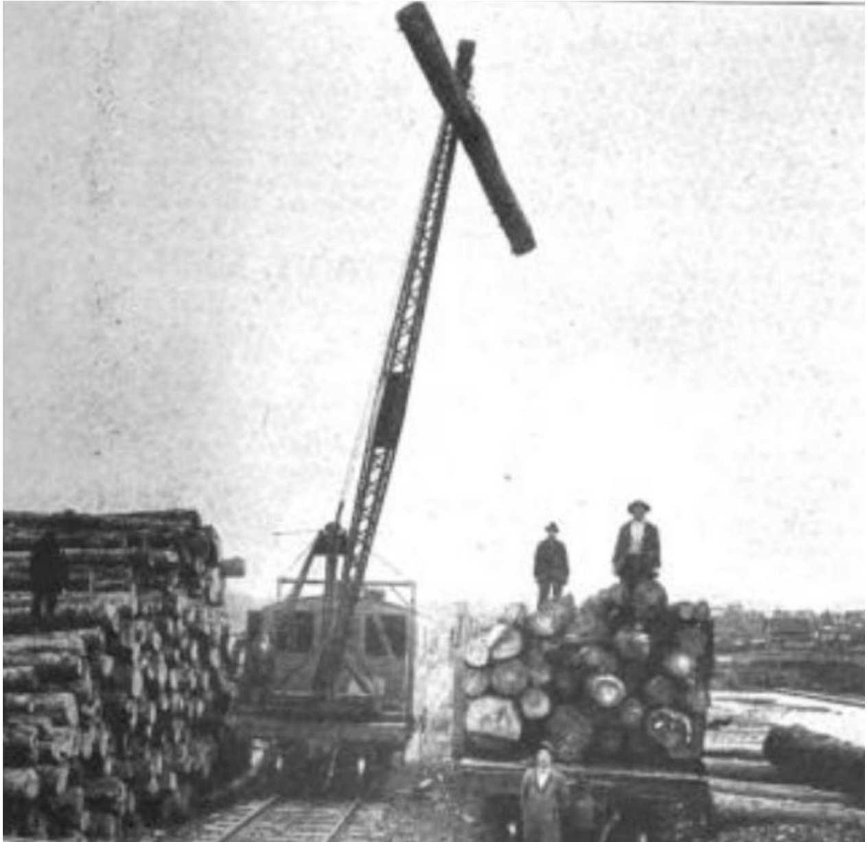
Figure D – 4. “Oval Wood Dish Co., Tupper Lake, N.Y. Raymond Gasoline Car Derrick does switching and general yard work. It is equipped with air brakes and electric lights.” 126
