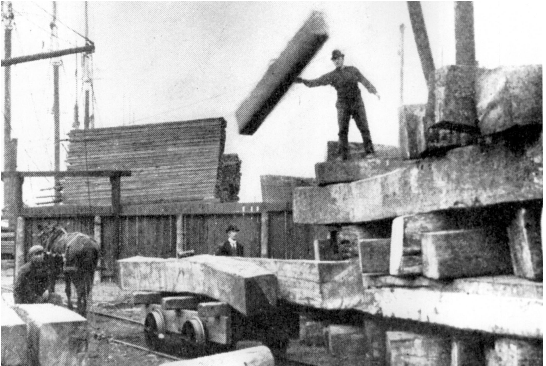
Figure G-8. "Small horse-drawn tram cars are used to move the large hewn logs around the manufacturing facility. Photo from The American Lumberman , May 23, 1903, courtesy of Mac Connery." 306
