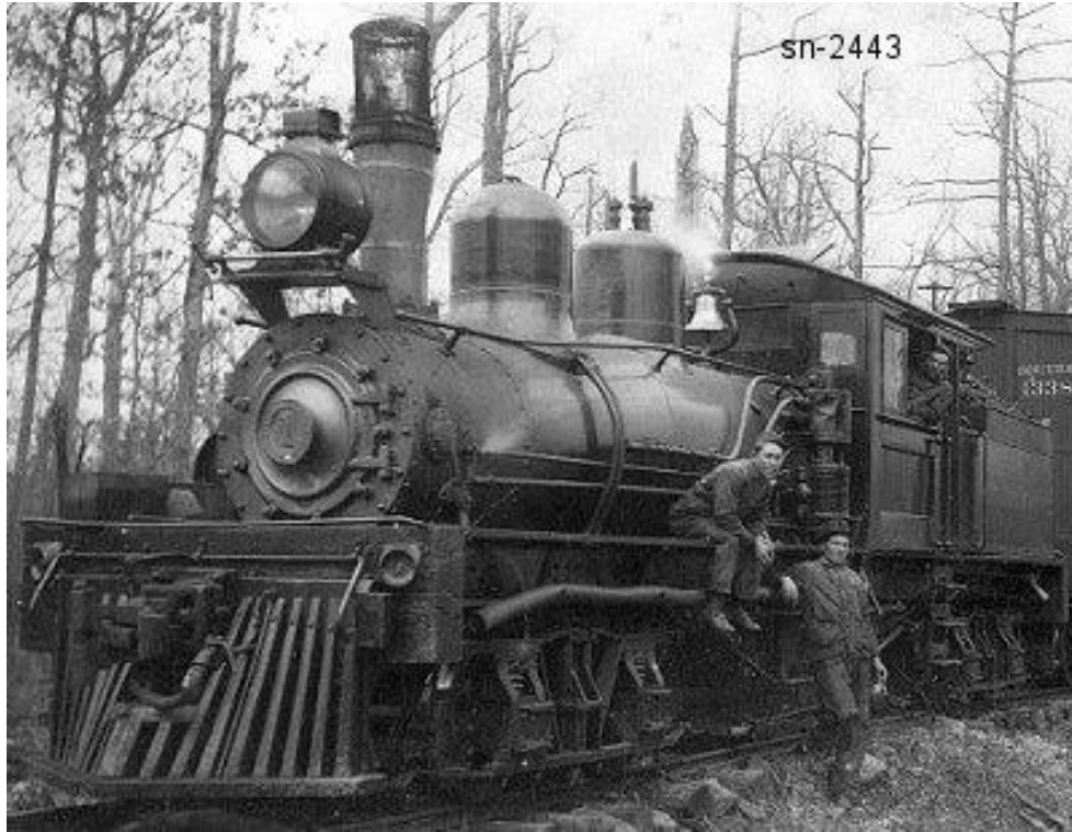
Figure D – 1. Greeneville & Nolichucky Railroad #1, a 42-ton Class B Shay, Shop Number 2443, that was built in 1911 for the John Heilman Lumber Company.
