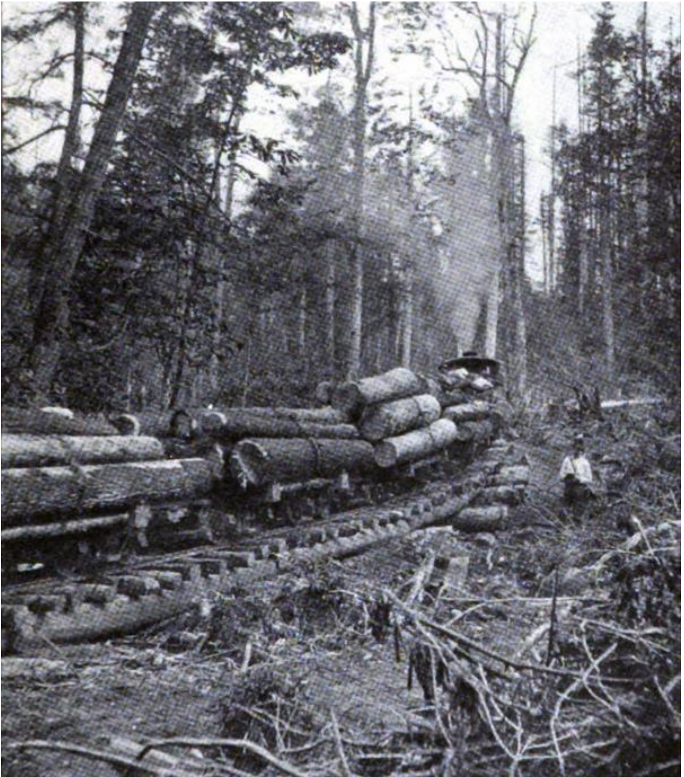
Figure 17. “Logging White Pine and Hemlock, Mitchell County” by 1911. 49 Author Thomas Feters captioned this photograph: “Tenuously perched on track built over a crude cribbing, the H.S. [should read H.L.] White Lumber Co. Shay No. 1 [Shop Number 2195] and four heavily-loaded log cars trundle south toward the White mill north of Elk Park, North Carolina. While the right of way still has slash obscuring the way, the big trees have been removed from the less mature in a non-clear cut harvest that allowed the forest to regain its stability. The technique of supporting the ties on long poles which in turn rested on transverse logs allows the line a more level right of way across the undulating hillsides above the Elk River. (Collection of R.D. ‘Doug’ Walker, Morganton, North Carolina)” 50
