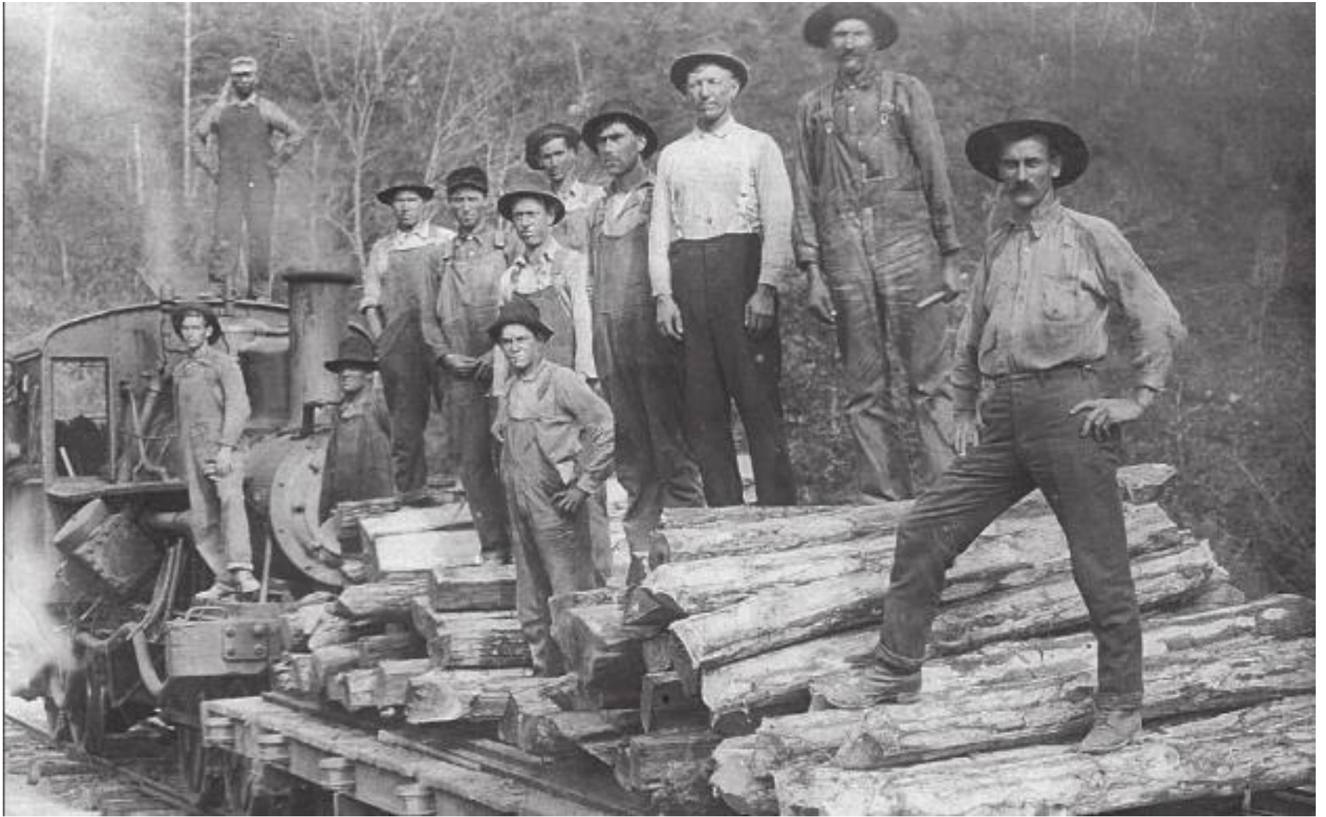
Figure 6. "Hauling Railroad Ties. Logging operations required miles of railroad track. These men are probably hauling railroad ties for the Valentine Lupert Lumber Company at Butler..." 19 Of note, the engine appears to be an otherwise unidentified Heisler locomotive.
