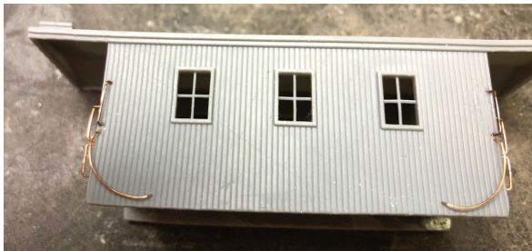
Unfinished 3D printed shell of caboose #503 with grabirons installed.
